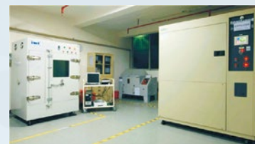
Natural convection test chamber (left), thermal shock test chamber (right)
